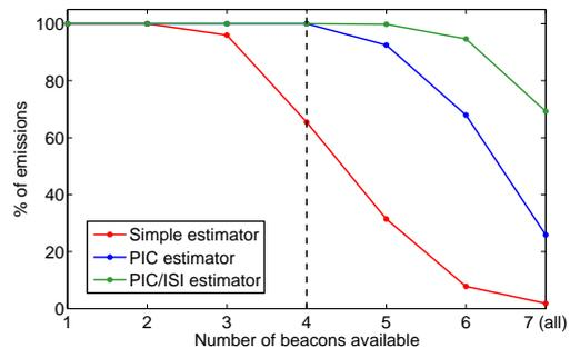
Fig. 7. Statistics with the number of beacons free of outliers and available for positioning, for three different CDMA estimators. The condition for System Availability (4 beacons are available) is shown with a vertical dashed line.
