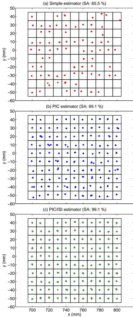
Fig. 8. CDMA performance of the positioning system over a  $11 \times 10$  grid with step 10 mm. Position computed with (a) the simple, (b) PIC, and (c) PIC/ISI estimators. Empty grid points correspond to regions where the System Availability condition was not reached.
