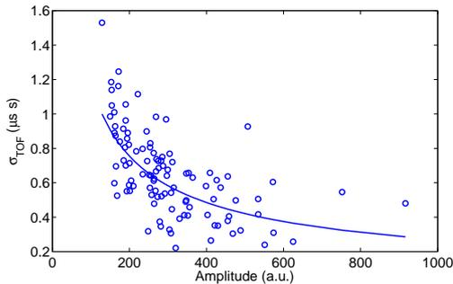
Fig. 3. The dispersion (standard deviation) of the times-of-flight from the acoustic beacons is inversely related to the received signal amplitude.
