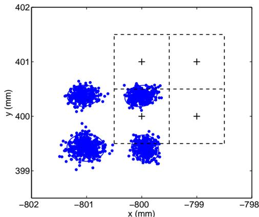
Fig. 5. Performance of the positioning system under reproducibility conditions. A positioning resolution better than 1 mm is obtained, but the measurement is affected by an error bias ( $b_x, b_y, b_z$ ) = (-0.9, -0.6, 0.7) mm.
