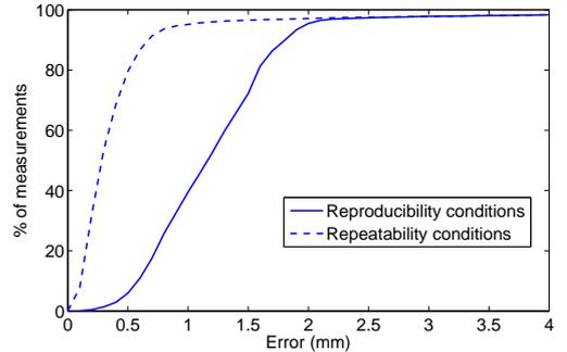
Fig. 6. Cumulative density function (CDF) of the positioning error of the acoustic system in TDMA operation. Reproducibility conditions encompass both systematic and dispersion errors, while repeatability conditions include only the dispersion error.
