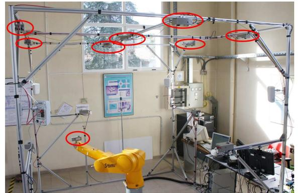
Fig. 1. The 3DLocus acoustic positioning system used in this work. The beacons of the emitting network at the top and the receiver (attached to the point of the robotic arm) are marked with red ellipses.
