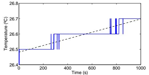
Fig. 2. Temperature variation during one of the experiments of section IV. We have improved on the limited resolution of the measured temperature (blue continuous line) by using instead a linear interpolation (dashed line).
