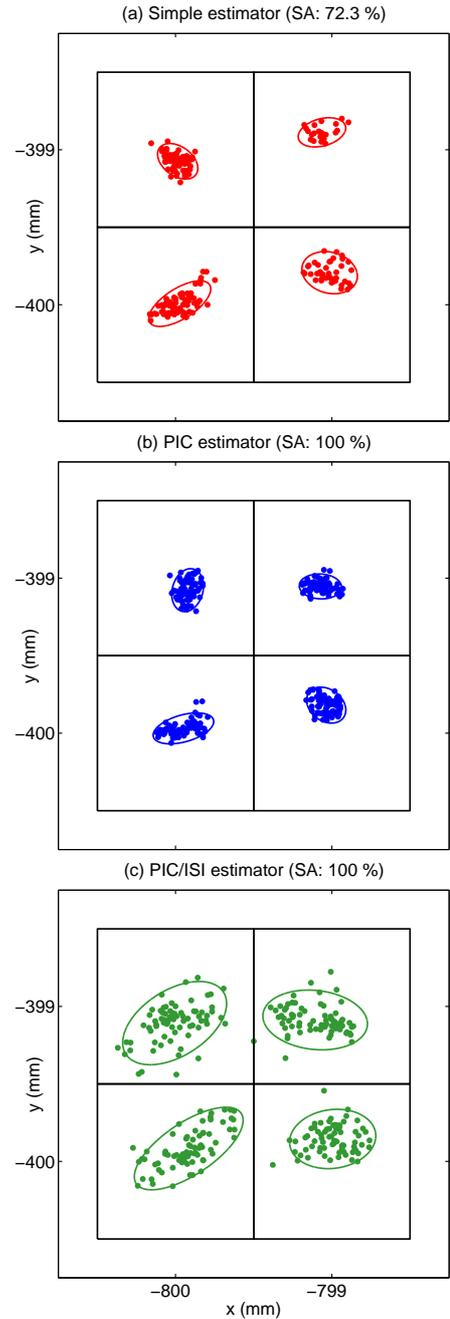
Fig. 9. CDMA positioning over a small  $2 \times 2$  grid of 1 mm size. Results of the (a) simple, (b) PIC, and (c) PIC/ISI estimators, and 90% confidence ellipses. Repeatability estimates with systematic error removed.
