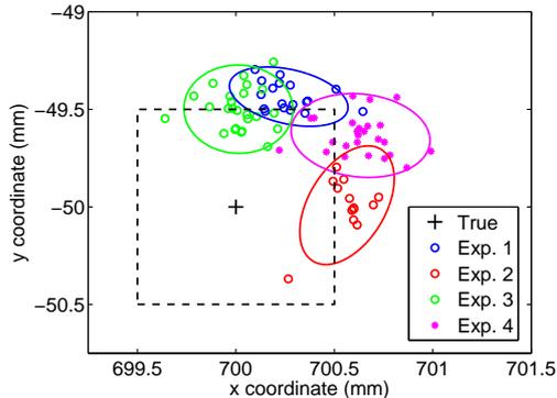
Fig. 4. TDMA positioning estimates ( $x, y$  coordinates) at point (700, -50, 600) mm in four different experiments carried at different times (reproducibility conditions). We include the 90% confidence ellipses and a 1 mm side square bound centered in the true position.
