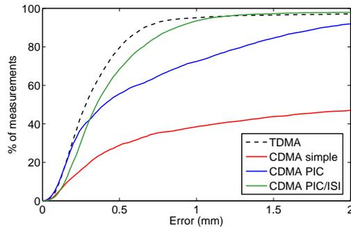
Fig. 10. CDF of the TDMA and CDMA positioning error results compared (under repeatability conditions, systematic bias has been removed).
