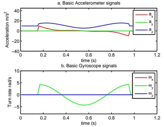
Fig. 4. Simulated accelerometer (a) and gyroscope (b) signal (in the body frame), using the basic trajectory for a foot-mounted IMU along a straight line walk, equations 1 and 2.
