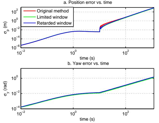
Fig. 8. Evolution of the root mean squared error over time (a. Position, b. Yaw) for the different step detection methods for an IMU signal with all the errors included
