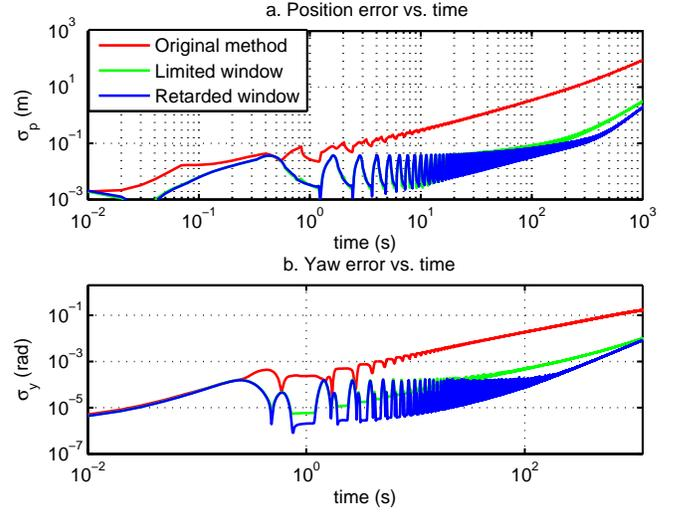
Fig. 9. Evolution of the root mean squared error over time (a. Position, b. Yaw) for the different step detection methods for an IMU signal with added accelerometer noise.
