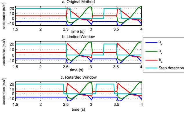
Fig. 7. Comparison of different stance detection methods for PDR INS/EKF mechanization: a. Original Method. b. Limited Window. c. Retarded Window
