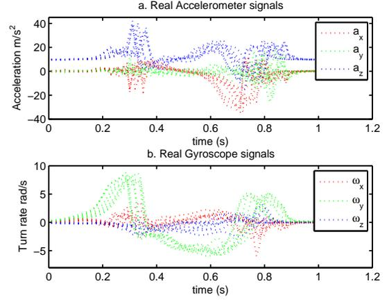
Fig. 3. Real accelerometer (a) and gyroscope (b) signals (in the body frame) of recorded steps from [1] rotated to have the gravity in the Z axis during the stance and move in the X axis.
