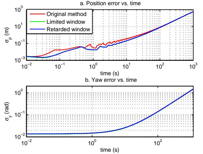
Fig. 10. Evolution of the root mean squared error over time (a. Position, b. Yaw) for the different step detection methods for an IMU signal with added gyroscope bias.
