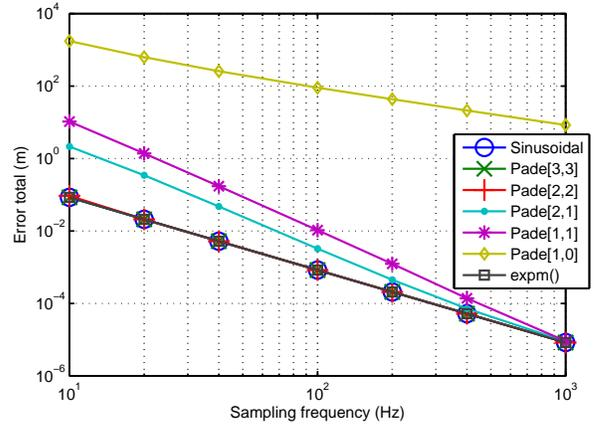
Fig. 6. Position error of an INS mechanization for different approximations for the attitude propagation. Study performed over a 10 step (13 m) straight walk with a basic pattern
