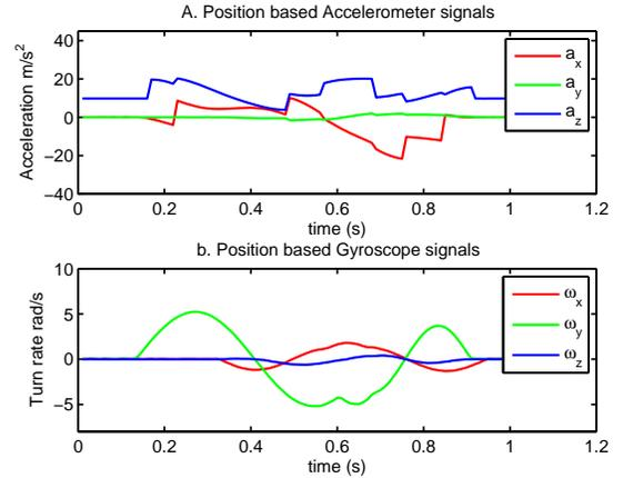
Fig. 5. Simulated accelerometer (a) and gyroscope (b) signal (in the body frame), using the fitted trajectory patterns for a foot-mounted IMU along a straight line walk, equations 3 and 4
