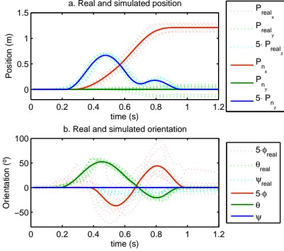
Fig. 2. Step patterns (a. Position and b. Attitude) detected with the Motion Capture System in [1] and the generated step patterns based on the minimization of the squared error.
