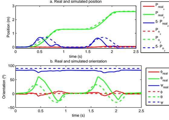
Fig. 1. Simulated two-step trajectory for a foot-mounted IMU and an equivalent trajectory obtained from a Motion Capture System in [1] (both in the navigation frame). a. Position vs. time ( $P_{n_z}$  is multiplied by 5 for an easier view) and, b. Attitude vs. time.
