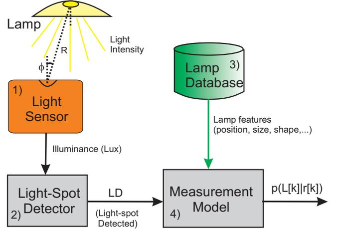
Fig. 5. Components in the measurement subsystem of the Light-matching approach: 1) Illumination sensor, 2) Light spot detector, 3) Lamp database, and 4) Measurement model.
