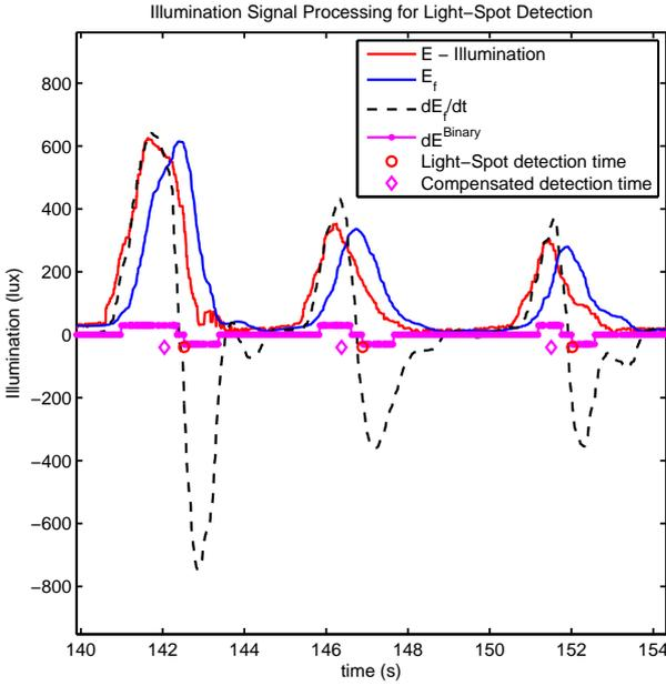
Fig. 6. Processing of the illumination data  $E$  to detect light spots. Real example for a person walking at constant speed in a corridor holding a smartphone (Samsung Galaxy S-3) on his hand.
