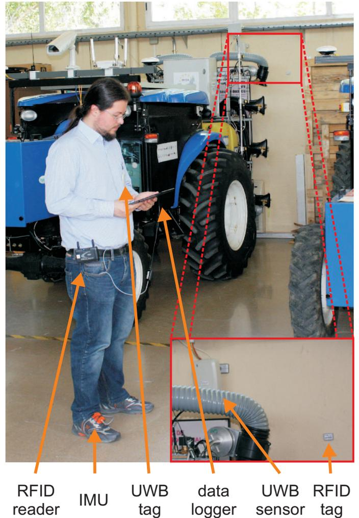
Fig. 5. Sensors used in the experiment, where it can be observed that one of the UWB sensors does not have a line of sight.
