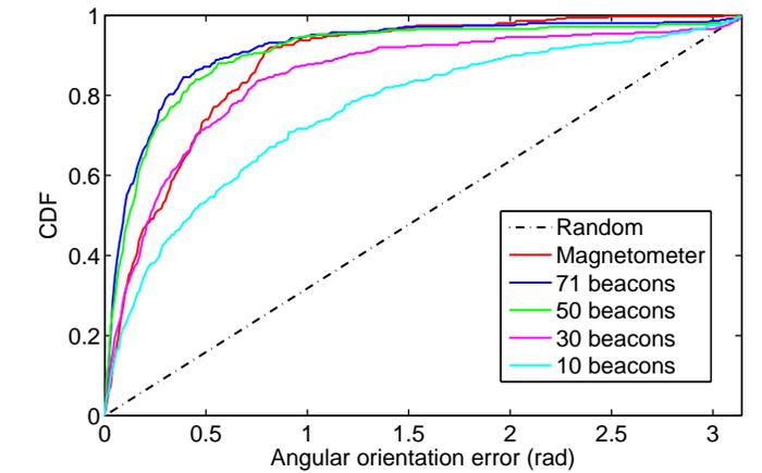
Fig. 12. CDF of angular error in dynamic trajectories versus number of active RF nodes.
