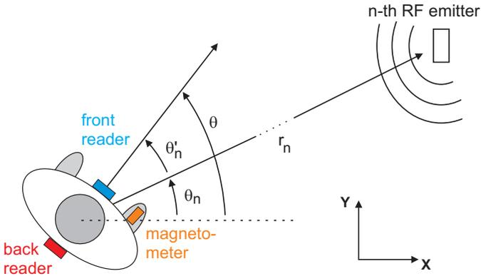
Fig. 1. Problem setup: a user receives an RF signal from an emitter with two readers placed in his front and back sides, and estimates its absolute angular orientation ( $\theta$ ).
