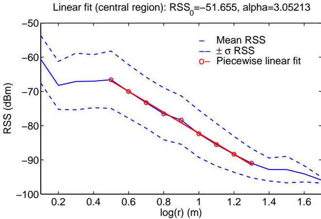
Fig. 3. Path loss law for for the calibration data of section III-B, without considering orientation.
