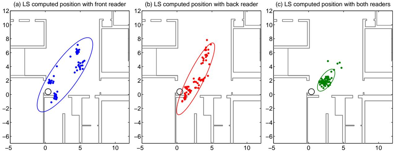
Fig. 7. The effect of orientation on the estimation of position, with only the front reader (a), the back reader (b), and both (c).
