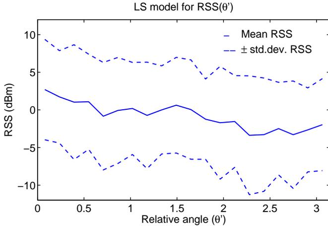
Fig. 4. Least squares model for the term  $RSS^{PL}(\theta')$  of Eq. 3, obtained from the calibration data.
