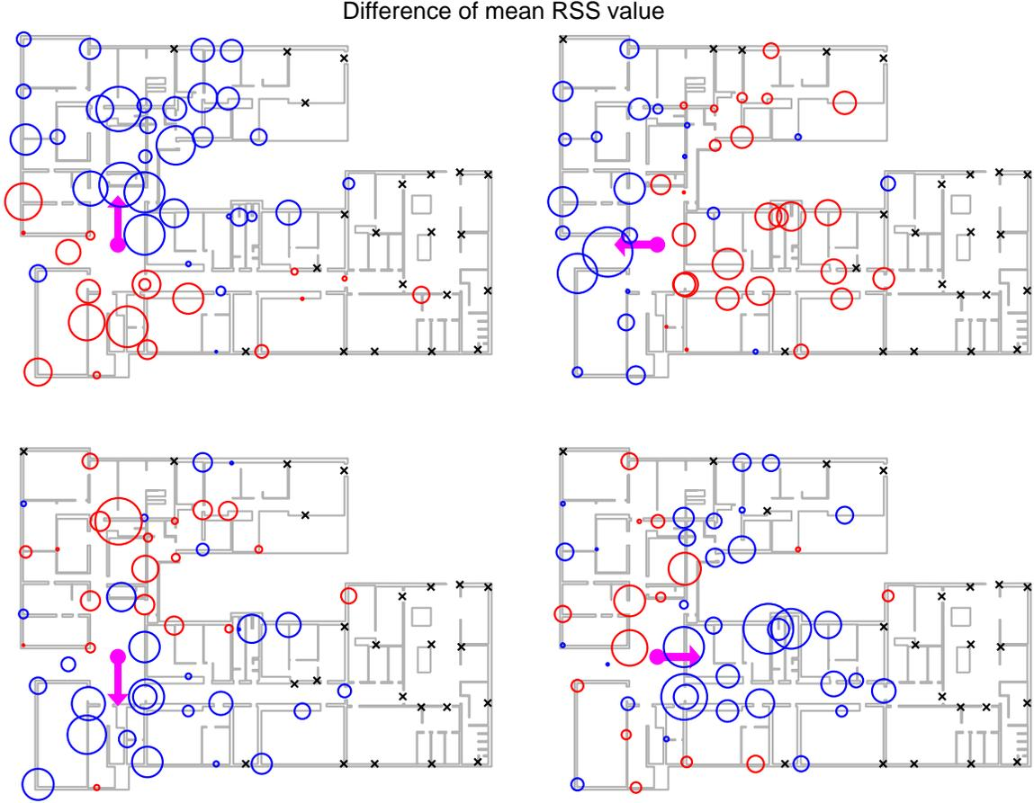
Fig. 2. Representation of calibration results when the user stands at one particular point (magenta full circle) with four different orientations (magenta arrows). The open circles represent the position of the tags and their sizes are proportional to the difference  $|\text{RSS}_n^{\text{front}} - \text{RSS}_n^{\text{back}}|$ ; they are coloured blue if the signal from the front reader is stronger, and red otherwise. Undetected tags are plotted as small black crosses.
