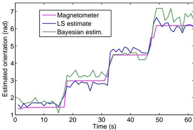
Fig. 8. Least squares- and Bayesian-based estimates of absolute orientation in the static setup described in part (c) of figure 7, compared with a foot-mounted magnetometer's readings.
