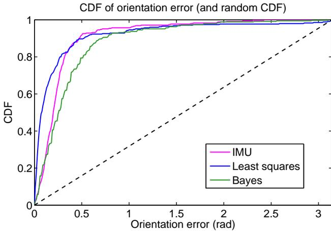
Fig. 11. CDF of angular error, as measured with the magnetometer, and computed through the least squares minimization and Bayesian estimation methods. The discontinuous line corresponds to the CDF of a purely random estimate of orientation.
