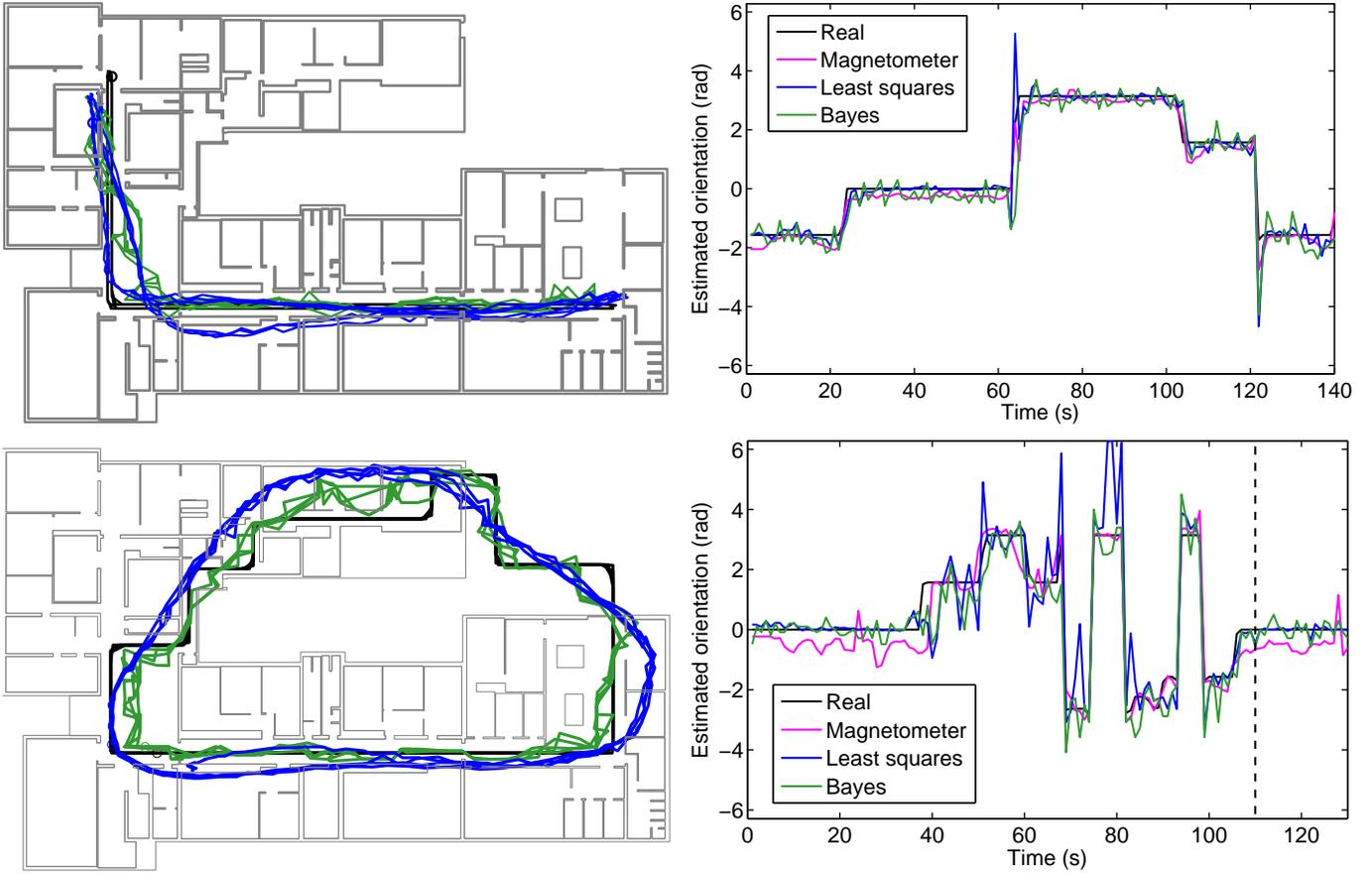
Fig. 10. Left column: two sample trajectories in our building; right column: absolute orientation determined from the heading of the trajectory, the magnetometer carried by the user, and by least-squares and Bayesian estimation (only one complete turn of each trajectory is shown).
