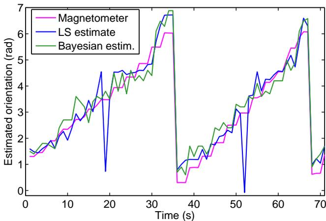
Fig. 9. A user turning around himself in counter-clockwise direction, at about 0.19 rad/s, and the estimated orientation by least squares minimization and the Bayesian method, compared with actual foot-mounted magnetometer readings.
