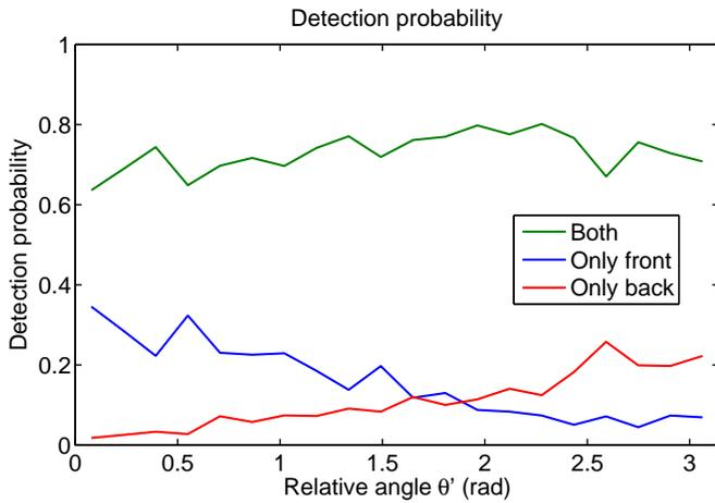
Fig. 5. Bayesian model for the detection probability of a given tag by the front, back, or both, antennas.
