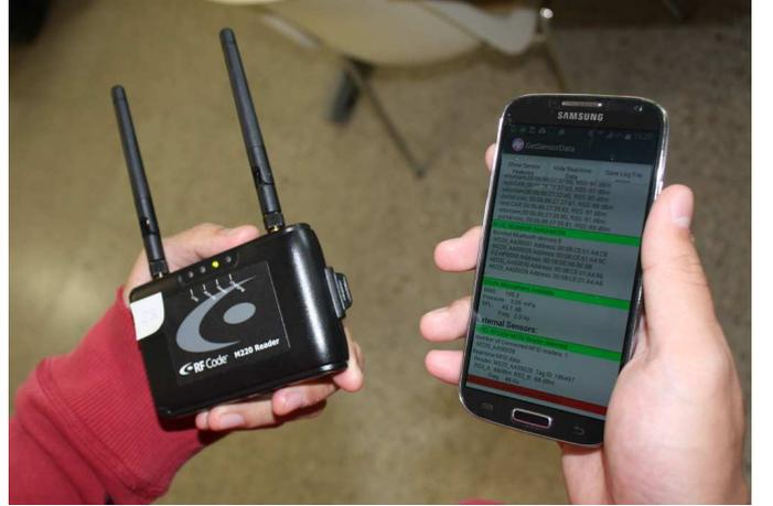
Fig. 1. Experimental device, formed by an RFID portable reader from RfCode (left) and a mobile phone (right) with dedicated software for data collection. Processing of the PF position estimation is performed offline.
