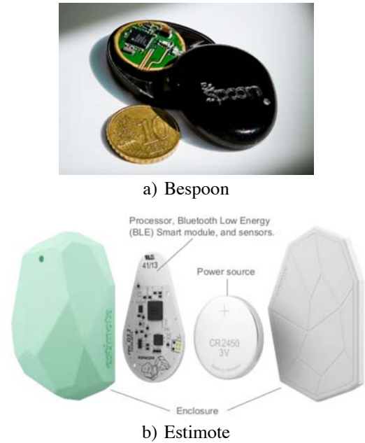
Fig. 1. Tags used for object finding in the museum-like use case. a) UWB tag from the Frech company BeSpoon, b) BLE tag from the Estimote company.
