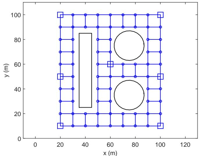
Fig. 2. Indoor testbed for evaluation of the MDS positioning methods. Nodes are arranged in a rectangular grid of step 10 m for this example. Square marks are anchor nodes with known location, circular marks are mobile nodes with unknown location. One rectangular and two circular obstacles impede node communication throughout them.
