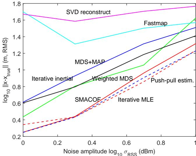
Fig. 6. Dependence of the RMS positioning error of the network, with the noise amplitude, obtained with an average of 10 simulations.
