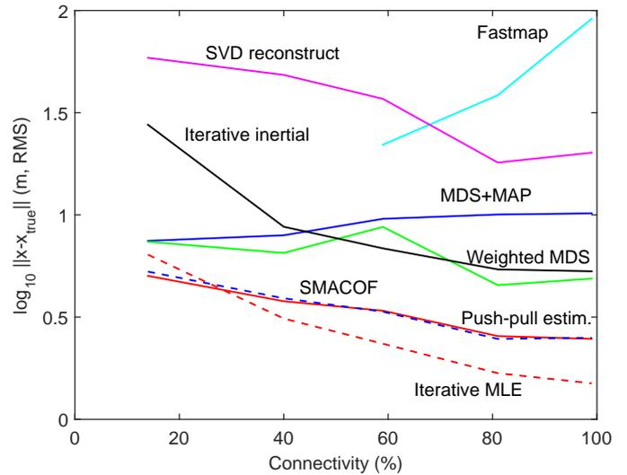
Fig. 5. Dependence of the RMS positioning error of the network, with the network connectivity, obtained with an average of 10 simulations.
