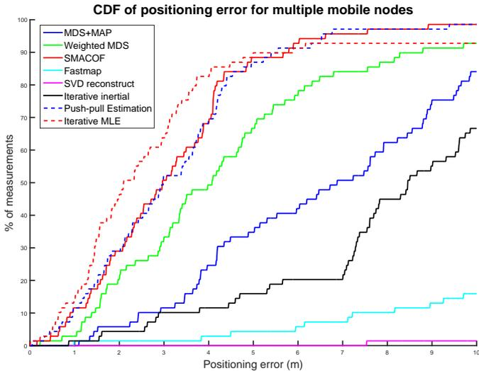
Fig. 4. Cumulative distribution function (CDF) of the positioning error of the estimated sensor arrangements of figure 3.
