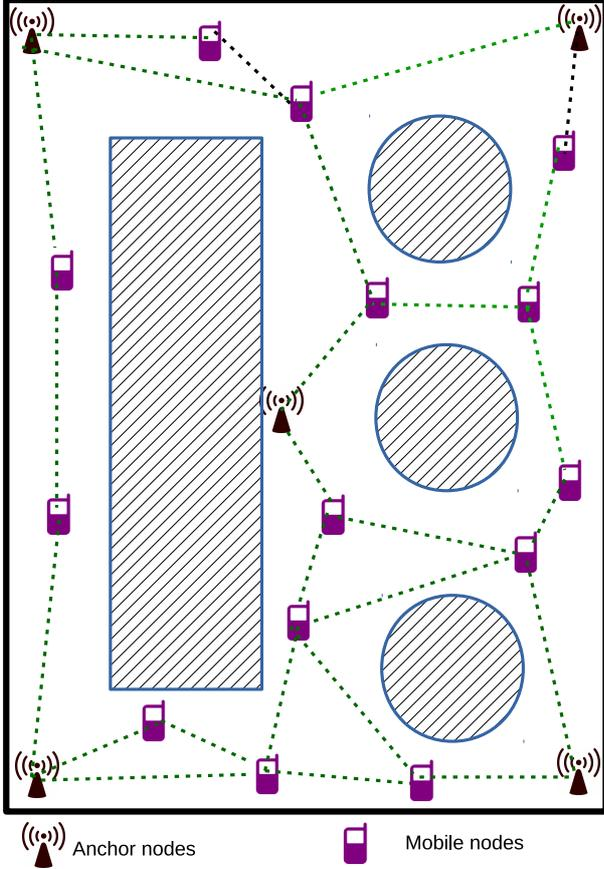
Fig. 1. Localization of the nodes of a wireless sensor network in an indoor environment. Anchor nodes have known positions, while mobile nodes have unknown positions to be determined. Neighboring nodes can measure the received signal strength of the RF signals exchanged between them (dashed lines).
