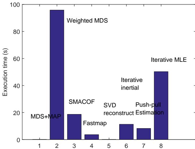
Fig. 7. Execution time of the MDS localization techniques of section IV as evaluated with Matlab.
