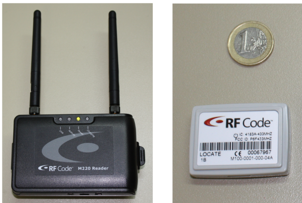
Figure 5: RFID reader (left) and tag used in the irradiation experiments, from the RFCode company.
