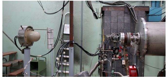
Figure 6: Arrangement of the batch of RFID tags in front of the output of the van de Graaff accelerator.
