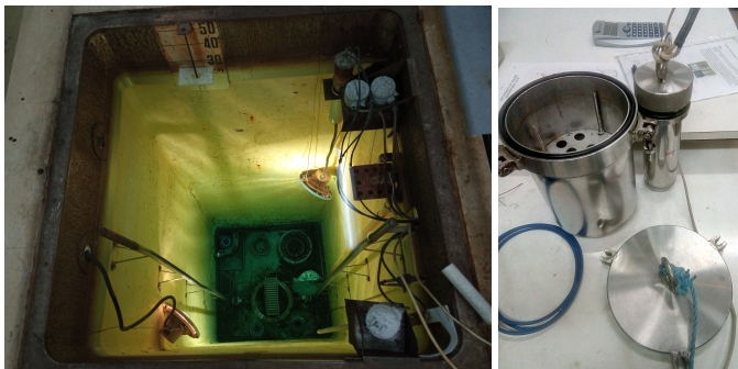
Figure 8: Image of the pool facility for gamma irradiation at CIEMAT (left), and sample holder to bring the electronic devices close to the radioactive sources (right).
