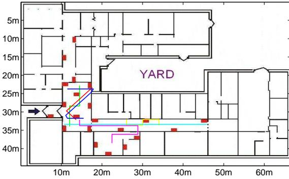
Fig. 3. FLOOR PLAN OF THE MAIN BUILDING OF THE INSTITUTE OF INDUSTRIAL AUTOMATION USED FOR THE EXPERIMENTAL TESTS. THE RED POINTS REPRESENT THE TAG POSITIONS. WE SHOW THE SIX ROUTES USED FOR EXPERIMENTAL TESTS (ROUTE 1: GREEN, ROUTE 2: BLUE, ROUTE 3: RED, ROUTE 4: CYAN, ROUTE 5: YELLOW, ROUTE 6: MAGENTA)
