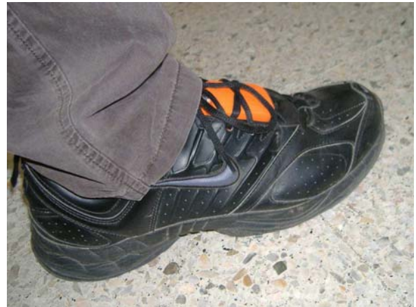
Fig. 2. Xsens IMU attached to the right foot using the shoe's laces.
