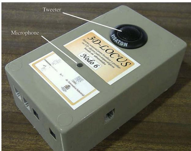
Fig. 6. Acoustic transducers (tweeter and microphone) installed in a 3D-LOCUS node.
