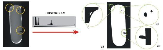
Figure 2. (Left) Intensity image and Histogram of a typical gob, (a) Binarized image, (b) Bright areas, (c) Dark spots, (d) Boundary holes
