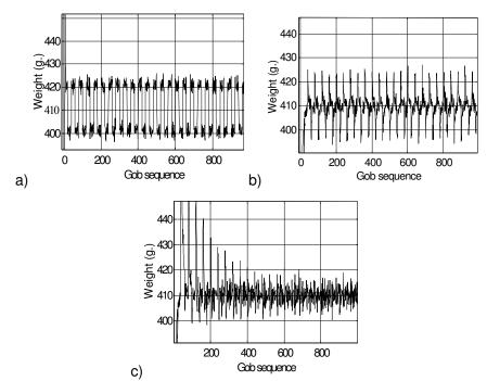
Figure 4.a) Open-loop response to a constant reference. b) PI control performance. c) PI-repetitive controls performance.
