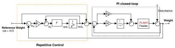
Figure 5. PI-repetitive control diagram
