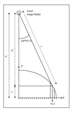
Figure 9. Drawing showing the parameters related in the correction of the distance to the
