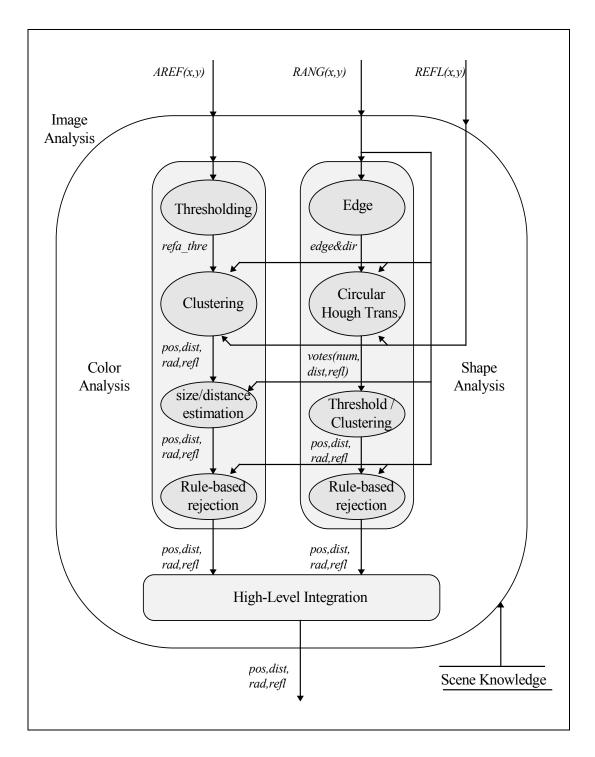
Figure 5. Data flow diagram of the dual image analysis approach. The left side represents the color analysis and the right side represents the shape analysis.
