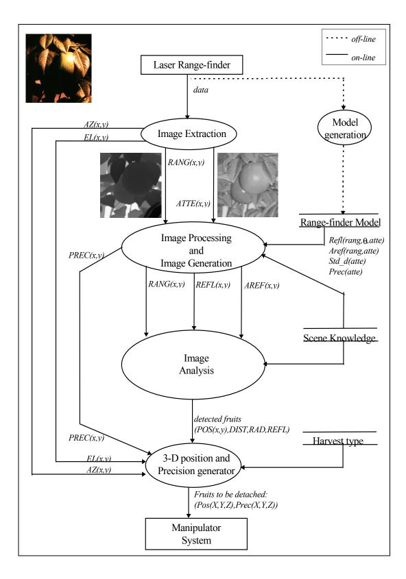
Figure 2. General Data Flow Diagram of the fruit detection process
