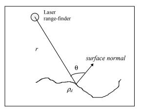
Figure 7. The angle  $\theta$  between the surface normal and the laser axis is necessary to obtain the
