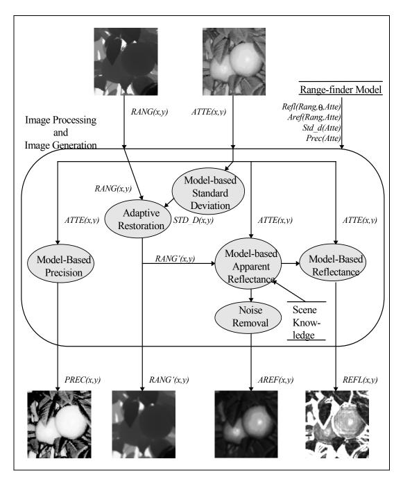
Figure 4. Data flow diagram of the image processing and image generation process. At the top are actual input images (RANG(x,y), ATTE(x,y)) and at the bottom, the output images (PREC(x,y), RANG'(x,y), AREF(x,y), REFL(x,y)).
