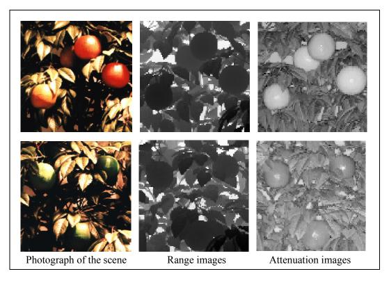
Figure 3. Some examples of range and attenuation images for two different artificial orange tree scenes. At the top, from left to right: scene with 4 mature oranges; the range image and the attenuation image. At the bottom, another sequence for a scene with 4 green oranges.
