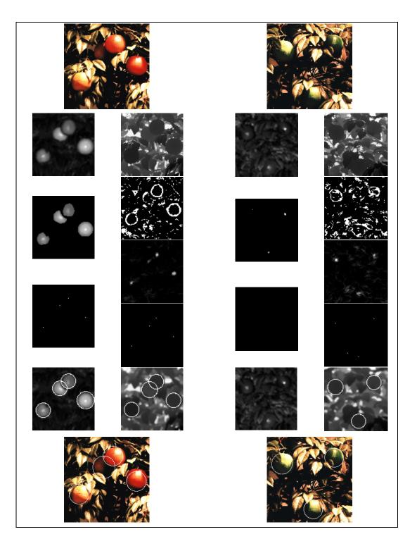
Figure 6. Some intermediate images during the image analysis process. At the top-left and top-right, two photographs are shown. Each of these images is processed by the color and shape analysis and the final results are displayed by overlapping circumferences with the computed radius.
