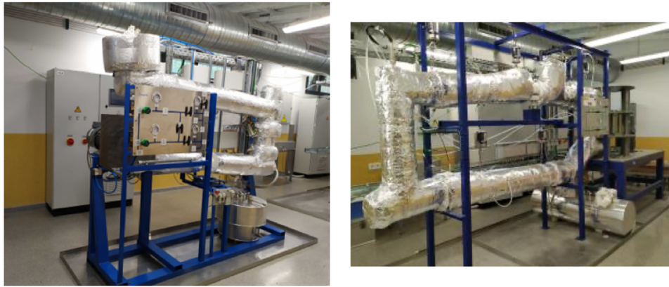
Fig. 8. On the left, a picture taken of CiCLO, the CIEMAT PbLi corrosion loop for testing of materials and corrosion protecting coatings. Also located at CIEMAT, the image on the right depicts CLIPPER, the PbLi loop designed for validation of permeation technologies.
